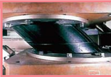
Seismic base isolation bearings
