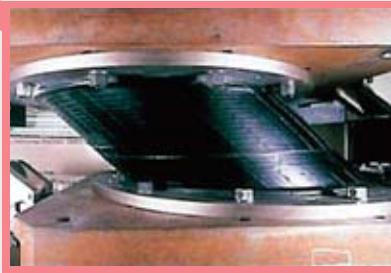
Seismic base isolation bearings
