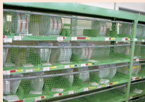
Nets to prevent inventory from falling off of shelves in case of an earthquake
